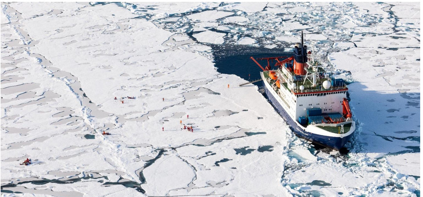
The German Research Icebreaker Polarstern (in English, “ Polar Star ”) has been the Alfred Wegener Institute's flagship since 1982. With a length of 118 meters, this 12 000-ton vessel is capable of sailing 300 days a year and wintering in the ice. Credit: AWI/Mario Hoppmann.
